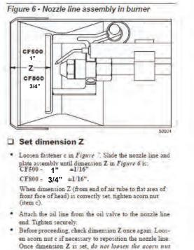
en acom nut c if necessary to reposition the nozzle line. Once dimension Z is set, do not lossen the acom nut (item) c again. Note that for the setting of fastener d, refer to Initial Head Position procedure on Page 11.
